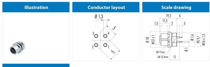
Contact arrangement (Plug-in side)
